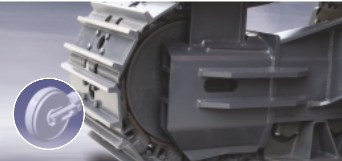
Integrated track spring and idler The track spring and the idler have been joined directly to achieve high durability and improved maintenance convenience.
